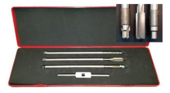
MPI melt pressure transducer/transmitter mounting hole cleaning kits are used to clean plastic residue from dirty or plugged holes before installing pressure sensors or extruder rupture disks. Hardened plastic residue is one of the leading causes of failures of melt pressure sensors or extruder rupture disks. The hardened plastic residue can damage the fragile diaphragm on the tip of the pressure sensors and extruder rupture disks, and can make them ineffective.
